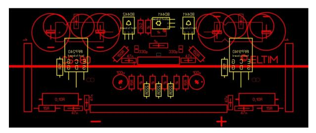
CS-80 preforming with normal polarity supply: left side is V-, right side is V+
