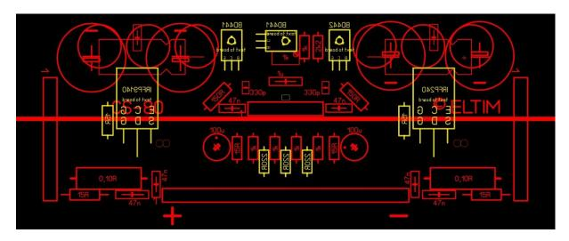
CS-80 preforming in reversed polarity mode where left side is V+, right side is V-
